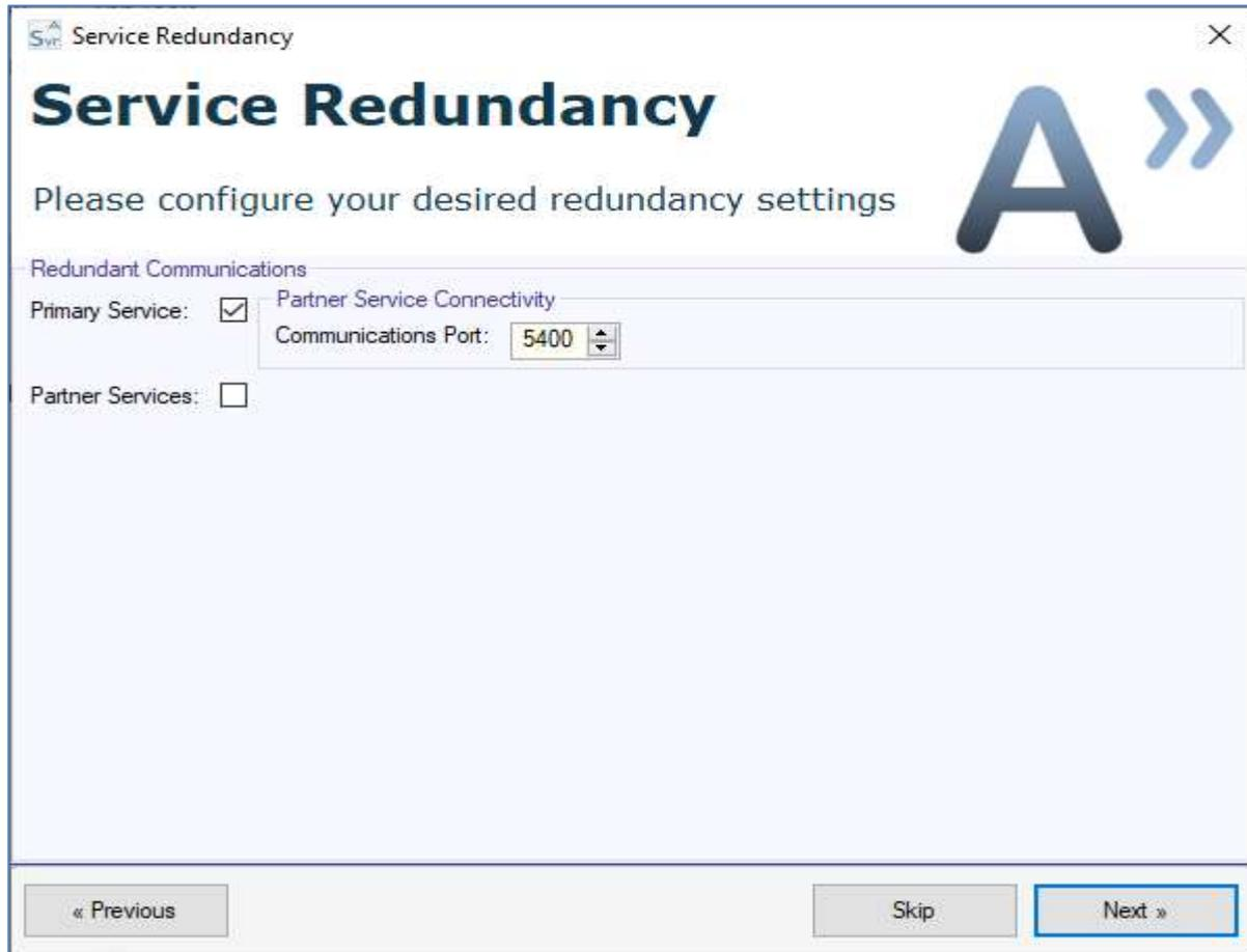
Select **‘Primary Service’** to enable Accord Server as a Primary service. It is not necessary to change the default **‘Communications Port’**, unless the internal network policy requires otherwise.
